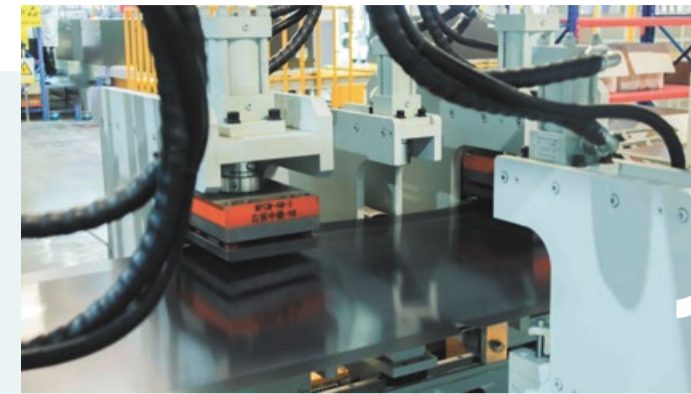
1 First step in producing the refrigerator side panel: punching and cutting the edges & corners of the metal sheet.
