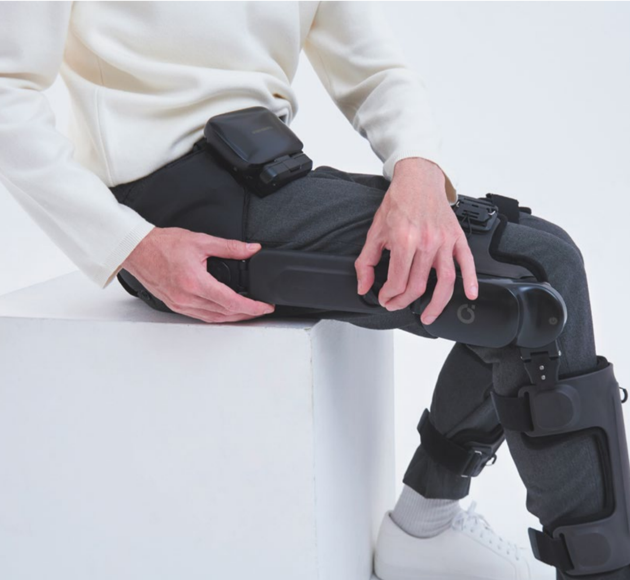
Angel SUIT wearable robot designed to support walking and encourage physical activity.
