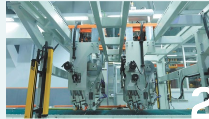
2 Final step in the side panel production process: attaching the condenser pipes to the formed panel.
