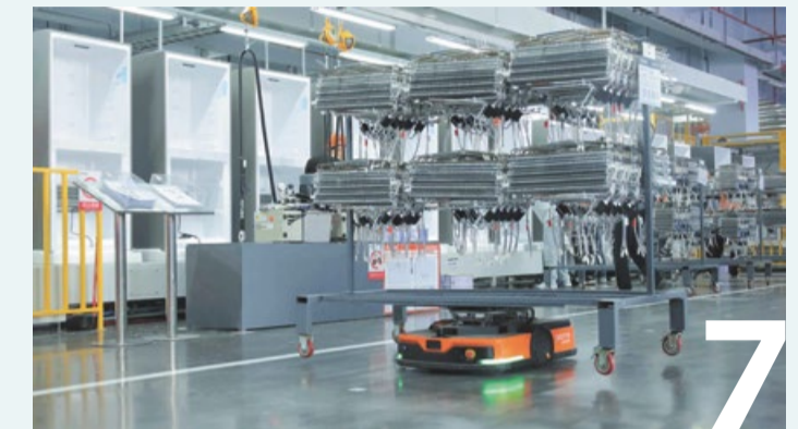
7 Smart, sensor-guided vehicles can move around without the need for an onboard operator.
