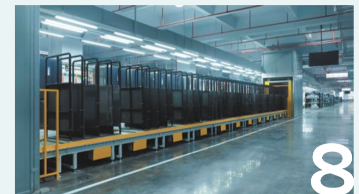
8 Once doors complete the pre-assembly and foaming stage, they are directed to the end of the cabinet assembly line.
