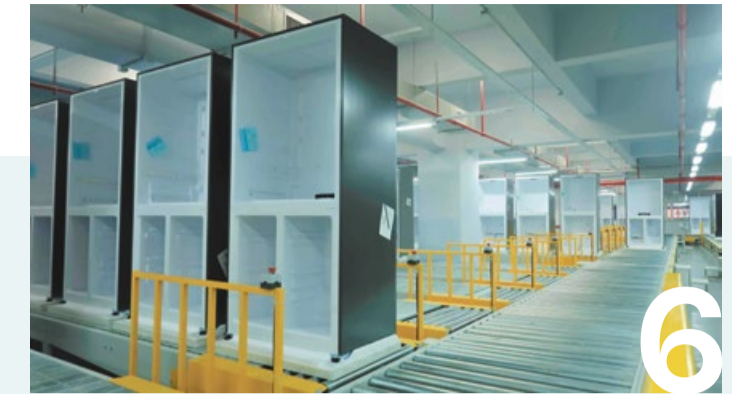
6 Automatic cabinet sorting identifies and directs the correct cabinets onto the final assembly line.
