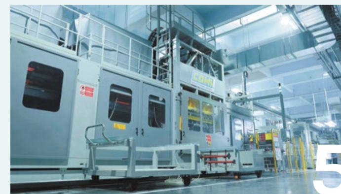
5 Vacuum-formed cabinet liners production process ensures speed and efficiency, supported by auxiliary hydraulic punching and shearing.
