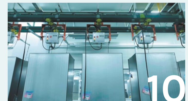
10 The dynamic cooling performance inspection line tests and ensures high cooling efficiency, allowing quick detection of any abnormalities.
